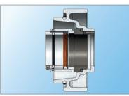
Encapsulated mechanical seal
