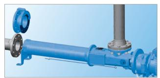
Step 1: Undo the connecting rod on the discharge flange side and push back, remove the discharge flange by lifting up.
