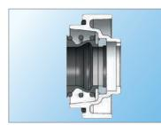
Mechanical seal with bellows
